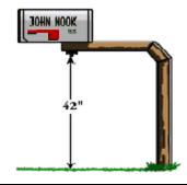
Mailboxes should be installed at least 42 inches high to provide clearance for the plow wing as shown in the picture on the right. We recommend the use of an extended arm type post with a free-swinging suspended mailbox as shown on the picture to the right. This allows snowplows to sweep near or under boxes without damage to supports and provides easy access to the boxes by carrier and customers.
